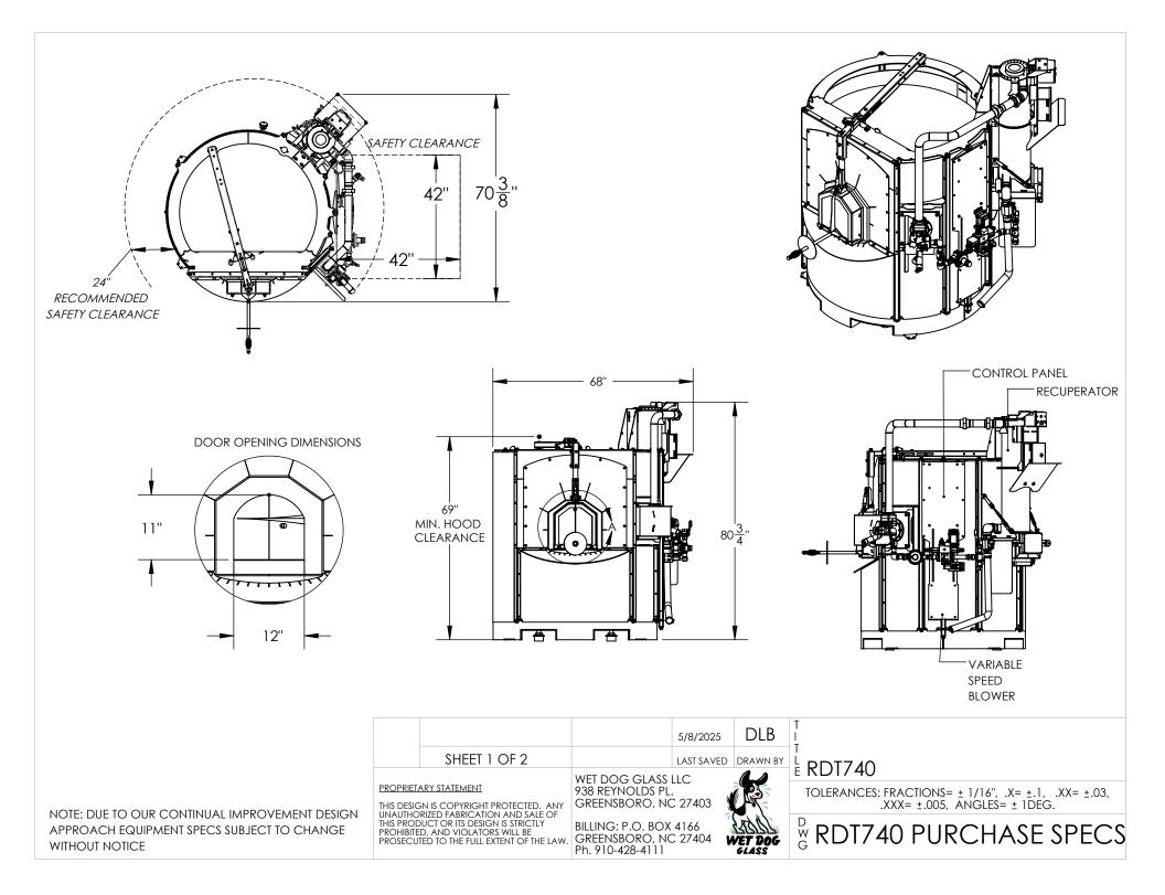
Model: RDT740 Capacity: 740 lbs Fuel: Propane/Natural Gas Fuel Pressure: 18"-28" w.c. Max Heat Output: 500,000 BTU/hr Air Supply: Variable Speed Blower Electrical Supply: 720 Watts. 120V for US, other voltages available Max Temperature: 2,450 F Exhaust Temperature: 2,000 F Equipment Weight: 5500 lbs Shipping Weight: 6050 lbs
