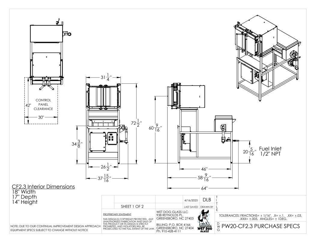
Model: CF2.3 Capacity: 2.3 cu.ft. Electrical Supply: ~5.5 kW (Available for most voltages, please specify voltage and phase) Max Temperature: 1600 F
