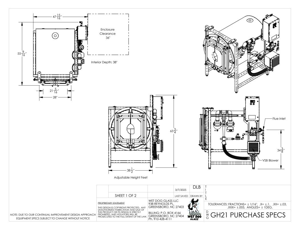
Model: GH21 Fuel: Propane/Natural Gas Fuel Pressure: 18"-28" Max Heat Output: 350,000 BTU/hr Air Supply: Variable Speed Blower Electrical Supply: 720 Watts. 120V for US, other voltages available Max Temperature: 2450 F Exhaust Temperature: 2000 F Equipment Weight: 1350 lbs Shipping Weight: 1450 lbs
