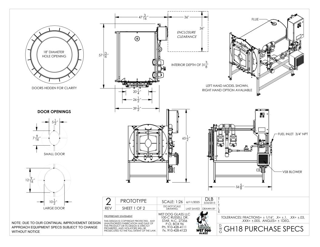
Model: GH18 Fuel: Propane/Natural Gas Fuel Pressure: 18"-28" w.c. Max Heat Output: 300,000 BTU/hr Air Supply: Variable Speed Blower Electrical Supply: 720 Watts. 120V for US, other voltages available Max Temperature: 2450 F Exhaust Temperature: 2000 F Equipment Weight: 1200 lbs Shipping Weight: 1300 lbs
