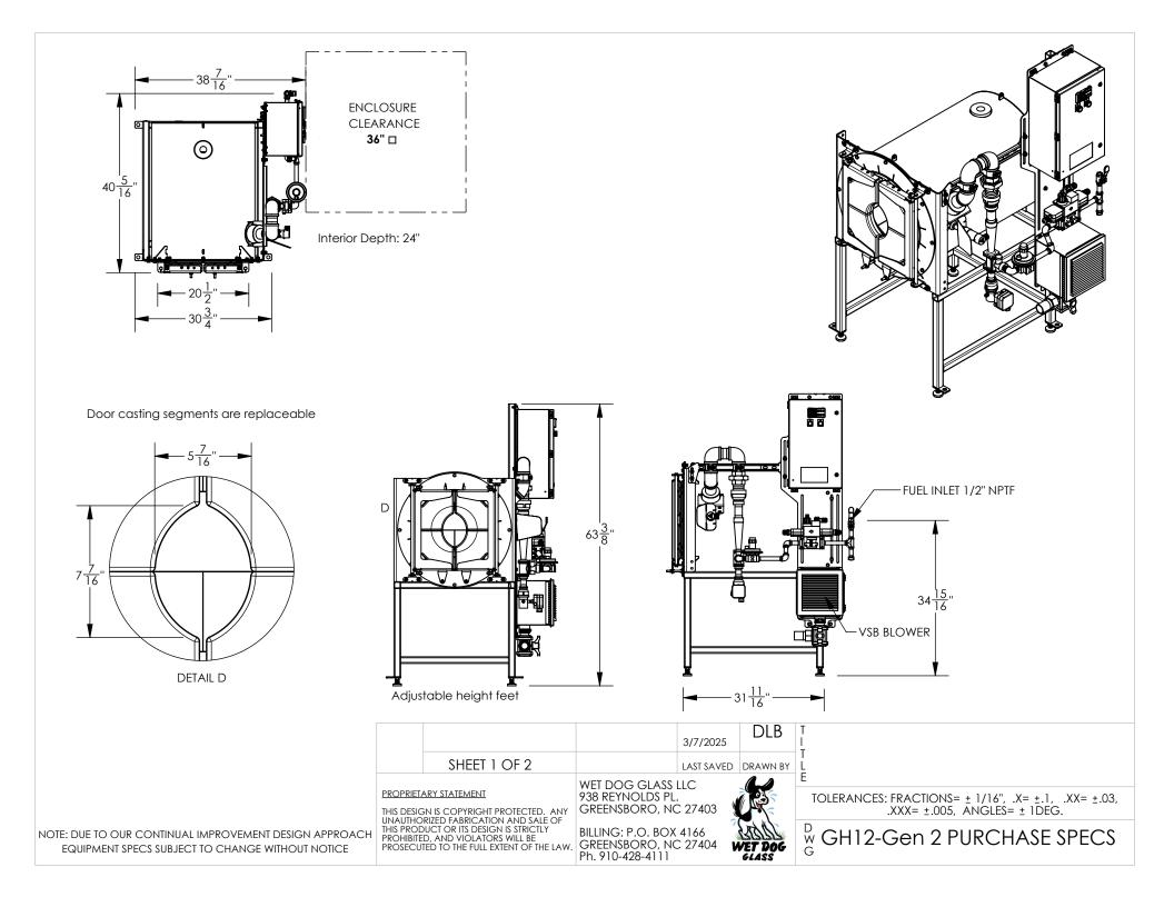
Model: GH12 Fuel: Propane/Natural Gas Fuel Pressure: 18"-28" w.c. Max Heat Output: 175,000 BTU/hr Air Supply: Variable Speed Blower Electrical Supply: 720 Watts. 120V for US, other voltages available Max Temperature: 2450 F Exhaust Temperature: 2000 F Equipment Weight: 800 lbs Shipping Weight: 900lbs
