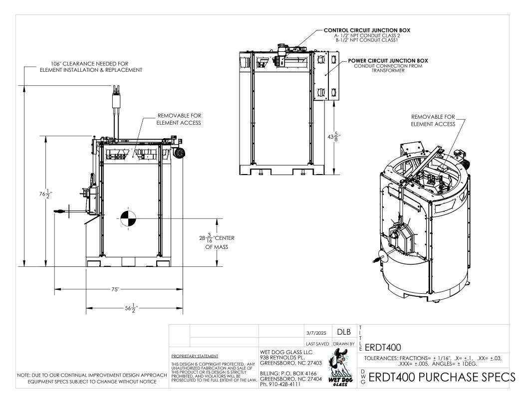
Model: ERDT400 Capacity: 400 lbs Electrical Supply: 27.6kW (Available for most voltages, please specify voltage and phase) Max Temperature: 2,450 F Equipment Weight: 3800 lbs Shipping Weight: 4000 lbs
